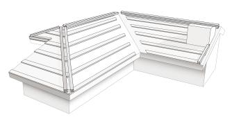
2"x2" ridge battens or double stacked 1"x4" pcs. are used to provide approximately 1½" of build-up height for hip and ridge pcs. Hip battens are installed directly on top of each intersecting panel bat-
