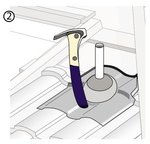
Slide the SMARTjack into place. Mold base of SMARTjack to conform with panel.
