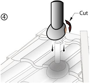
For added protection and appearance, SMARTsleeves are cut to conform to the panels and are installed over pipes. Sleeves are fastened with a screw through the front of the SMARTsleeve into the SMARTjack.
