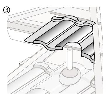
Measure, mark, and cut Roman panels to cover back section of SMARTjacks. Seal around flashing.
