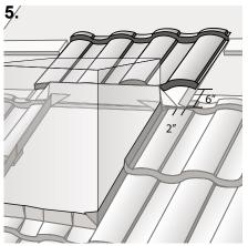
Apply a bead of sealant across Foam Closure and 'Seat' back cut-section panel onto Foam Closure. Panels are fastened through the front downturn of the panels, the Foam Closure and saddle into decking.
