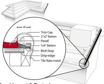
Metro Tile Rake metal is installed along the rake edges as shown. Tile Rake metal aids in positioning Metro Trim Caps, and is placed on the wood build-up. The Metro Trim Caps cover battens and folded up Metro panels, as shown.
