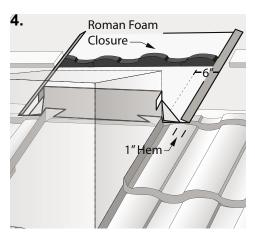
At back of chimney, install chimney saddle as shown. Extend saddle a minimum of 6" past each side of chimney. Hem ends 1" to keep water on saddle flashing. Install a section of Metro Roman Foam Closure across the chimney saddle as shown (align with Roman profile).
