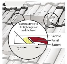
Where applicable, cut and fold panels to overlap the hand fabricated hem on the sides of the chimney saddle.
