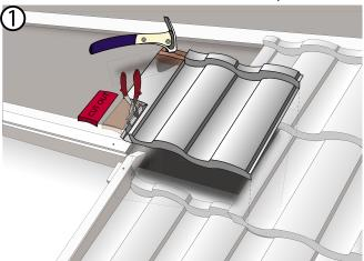
Where panels intersect with a stepped fascia, stop panel battens approximately 6" away from new fascia line. If nessesary, notch, cut, and flatten panel at this intersection as shown.
