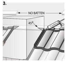
At back of chimney, seal each top corner section. Keep panel battens away from saddle as shown.
