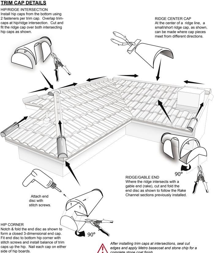
edges and apply Metro basecoat and stone chip for a complete stone coat finish.
