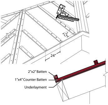
1"x4" counter battens are placed approximately 24" o/c directly over rafters. Fasteners must penetrate 1" into or through the roof framing members and be placed 12" o/c.
