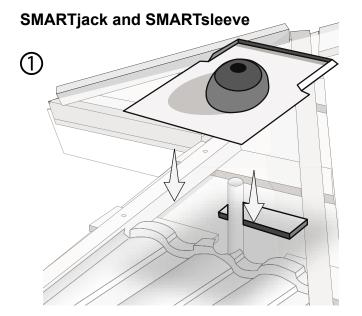
Cut panel battens a min. of 6" from the protruding pipe. Flatten the panel directly below the pipe to avoid a hump. Cut and hem a lip around the perimeter of the SMARTjack on the section placed above the panel batten. Install a block behind the protrusion to support the back of the SMARTjack.
