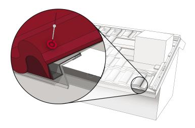
Fasten the first course of panels at the raised panel section, through the fascia metal, and into the 1"x4" batten. This is the only place where it is acceptable to fasten panels through the top.
