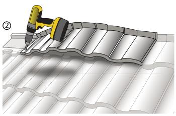
Then fasten panels at bottom far left corner. Panels are then pushed down and fastened into place.
