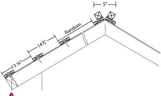
Wood panel battens can be 2"x2", 1"x3" or 1"x4". Consult Metro regarding approved steel purlin sections. Precise panel batten spacing is critical because the rear of each Metro panel must fit snuggly against the batten.
