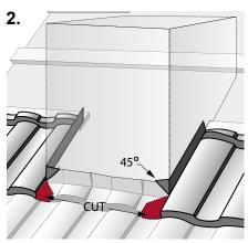
On sides of chimney, cut and fold up panels 2" as shown.
