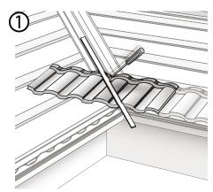
Measure, mark and cut panels to fit tightly against valley center (reverse 'V'). Fasten valley section panels to roof decking similar to the other panels without penetrating valley flashing.
