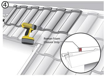
Install full panels aligned with main courses. Fasten with screws, through front down-turn of panel through the Foam Closure strip, and into the panel below as shown.
