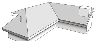
Metro Roman Tile panels are Installed on new or existing roofs pitched a minimum of 2-1/2:12 (12 degrees). An underlayment is to be installed as per local code and manufacturers instructions.
