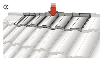
Push back of panel into position against ridge batten before fastening.
