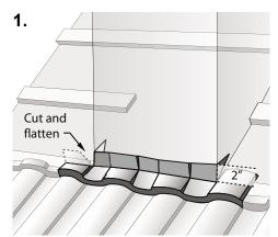
At front of chimney, measure, cut, and fold up panel 2". Cut panels on a 45 degree angle as shown and fold tabs around chimney.
