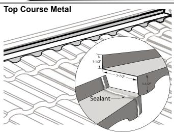
Roman Top Course metal may be used to avoid bending and cutting full panels at the ridge or chimney.
