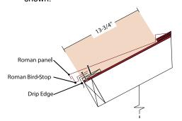
The Bird-Stop riser metal creates a 3/4" off-set from the fascia. The use of this 'Bird-Stop' requires standard Drip-Edge metal to be installed on a (1"X4" or 2"X2") support batten.
