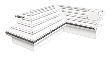
A standard "Drip-Edge" flashing is used along the eave/fascia, and should be installed over the batten, as shown.
