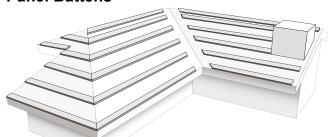
1"x4" or 2"x2" panel battens may be used over a solid sheathed roof deck. For installation using 1"x4" counter battens, 2"x2" panel battens must be used (see Counter Battens). Panel battens are installed parallel to the ridge/fascia. The first panel batten is positioned flush with the fascia or batten build-up. The second panel batten is positioned 13-3/4" from the fascia to accommodate the "Bird-Stop" metal.
